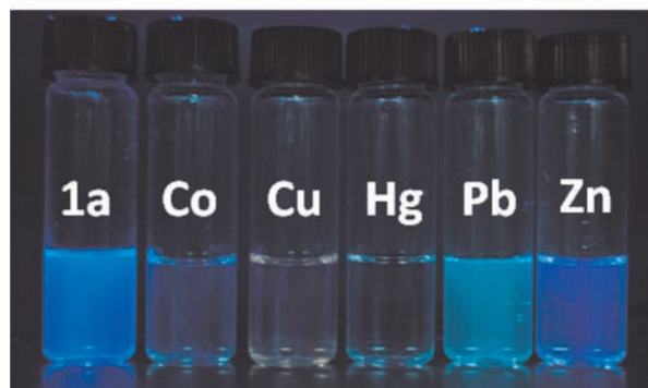
Figure 3. Fluorescence spectra of 1a (10 \mu\text{M} ) and upon addition of ClO 4 - salts of Hg 2+ , Pb 2+ , Cu 2+ , Zn 2+ , and Co 2+ (10 equiv, each) in CH 3 CN with an excitation at 305 nm (upper). Visual appearance of solutions of 1a with the above metals, under UV-light (lower).
